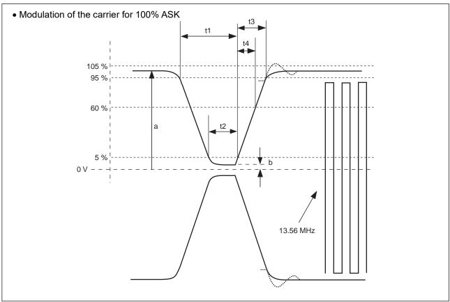
Maximum and minimum values of t1, t2, t3 and t4 are shown in the table of "■ RECOMMENDED OPERATING CONDITIONS". In this table, y is 0.05 (a-b) and the maximum value of hf and hr is 0.1(a-b).
