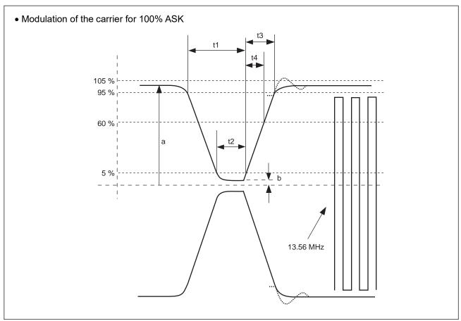
Maximum and minimum values of t1, t2 and t3 are specified in "RECOMMENDED OPERATION CONDITIONS". y is 0.05 (a-b) and the maximum value of hf and hr is 0.1(a-b).
