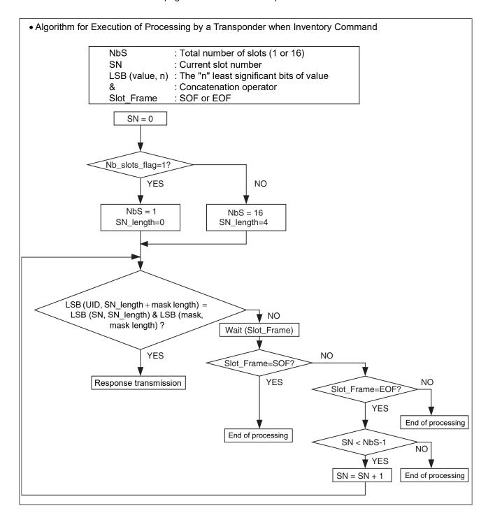
• Principle of comparison between the mask value, slot number and UID
