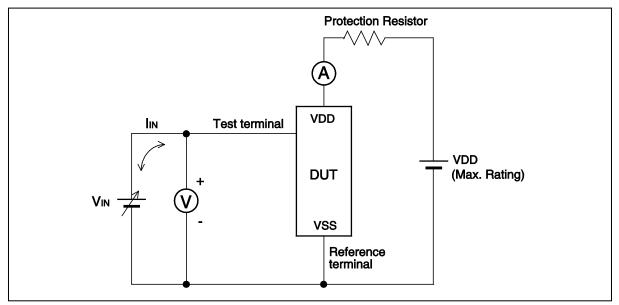
Note: The voltage VIN is increased gradually and the current  $I_{IN}$  of 300 mA at maximum shall flow. Confirm the latch up does not occur under  $I_{IN} = \pm 300$  mA. In case the specific requirement is specified for I/O and  $I_{IN}$  cannot be 300 mA, the voltage shall be increased to the level that meets the specific requirement. - C-V method of Latch-Up Resistance Test
