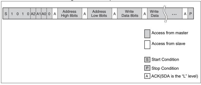
Note: It is not necessary to take a period for internal write operation cycles from the buffer to the memory after the stop condition is generated.
