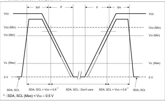
When applying relatively short term  $V_{DD}$  pulse whose peak is more than 1.6V, it is required to set falling time, tf more than 0.4ms/V. (In case  $V_{DD}$  rises over 1.6V and falls just after that, if this term is short, device may lose its function.)
