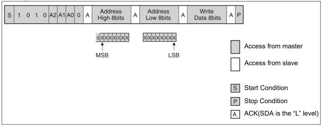
Note: In the MB85RC256TY, input "0" to the most significant bit of the higher address byte because the address is expressed with 15 bits.
