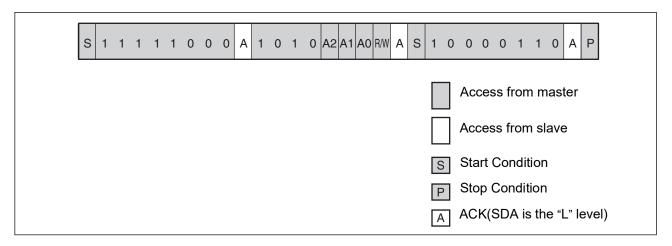
Even if the MB85RC256TY stays in the Sleep mode, SDA and SCL signals are monitored. Following sequences enable the transition to Standby mode after recovery time (tree) of internal regulator circuits.
