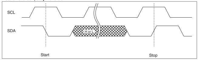
Note: At the write operation, the FeRAM device does not need the programming wait time (twc) after issuing the Stop Condition.
