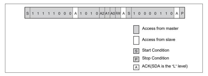
Even if the MB85RC512TY stays in the Sleep mode, SDA and SCL signals are monitored. Following sequences enable the transition to Standby mode after recovery time (tree) of internal regulator circuits.
