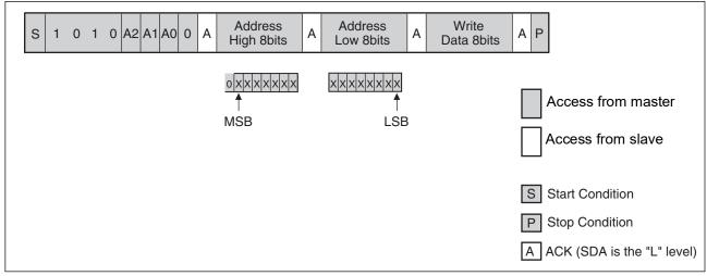
Note: In the MB85RC256VN, input "0" to the most significant bit of the higher address byte because the address is expressed with 15 bits.
