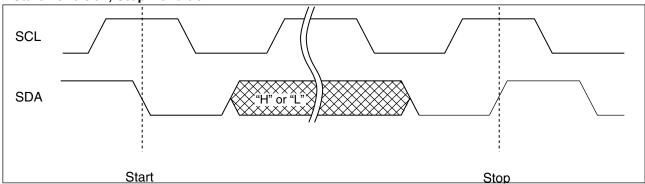
Note: At the write operation, the FeRAM device does not need the programming wait time (twc) after issuing the Stop Condition.
