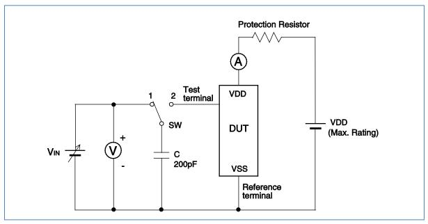
Note: Charge voltage alternately switching 1 and 2 approximately 2 sec intervals. This switching process is considered as one cycle.
